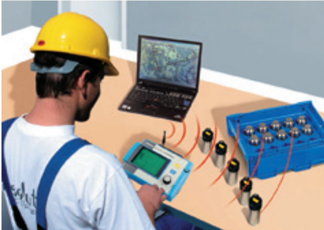
Reading and programming of loggers with radio link, analysis of data by PC
